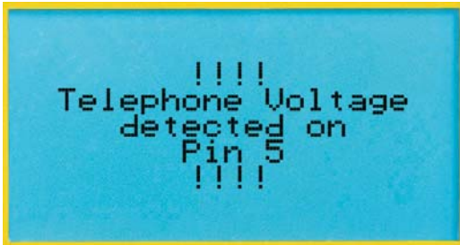
Automatic detection of live telephone voltage.
