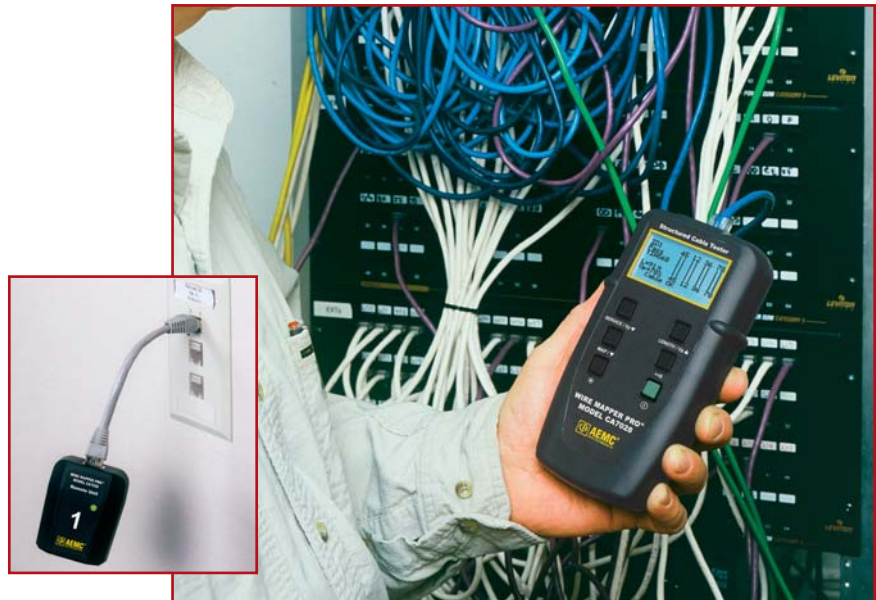
Model CA7028 used to locate and test a cable from the patch panel to an office a few hundred feet away.
